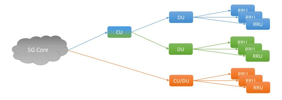
CU: Centralized Unit DU: Distributed Unit RRU: Remote Radio Unit
