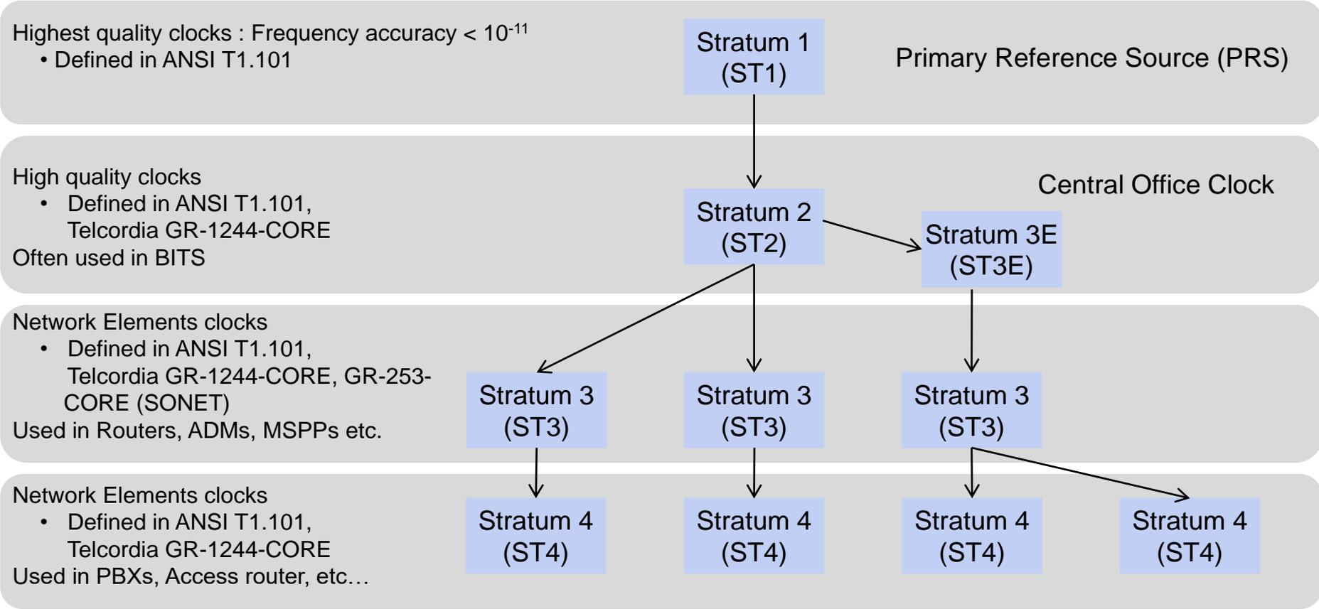
BITS – Building Integrated Timing Supply
