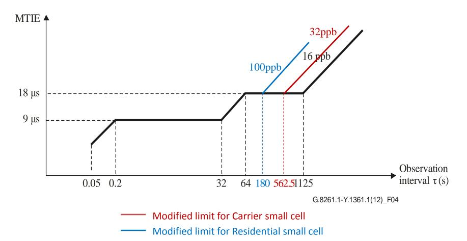
Figure 4/G.8261.1 – Output wander network limit for case 3 based on [ITU-T G.823]
