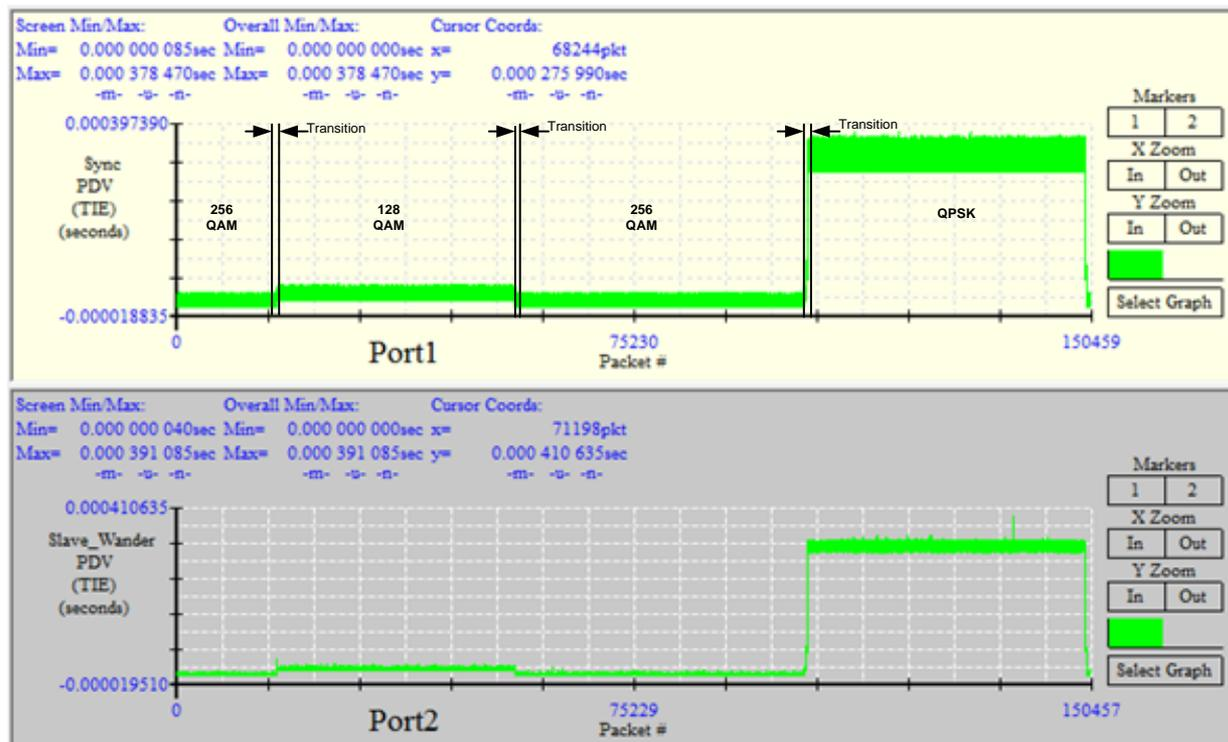
Figure 3: PDV TIE per Packet Response for: QAM256 to QAM128 to QAM256 to QPSK to QAM256
