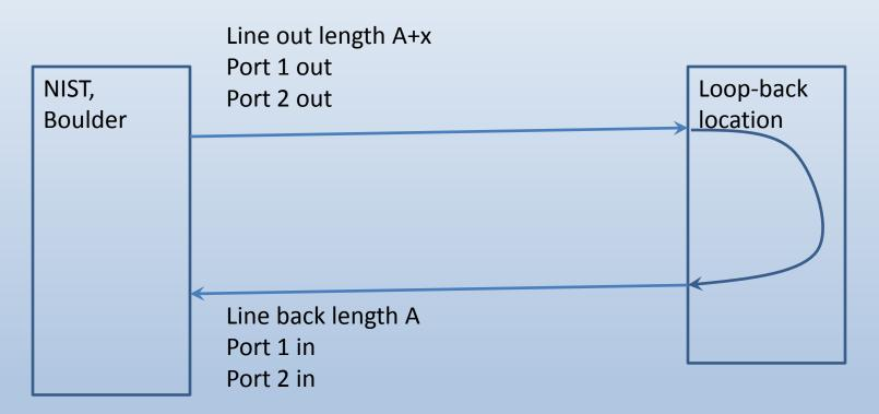
For loop-back we are emulating time transfer between two locations by using two ports on the same device in NIST. Both the loop from Port 1 and from Port 2 measure a delay of 2A+x, hence the difference between length A and length A+x is not seen.
