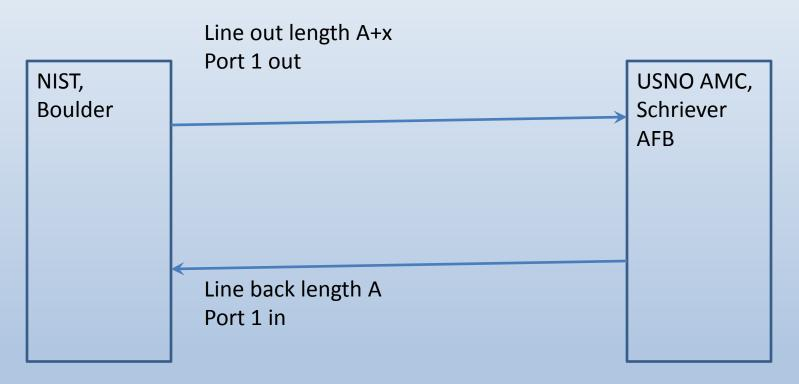
Because NIST and USNO both have UTC synchronized within 10 ns, we measure the one-way delays in each direction. We see the difference x between the path of length A+x and the path of length A. We have seen a differential x of 40  $\mu$ s.
