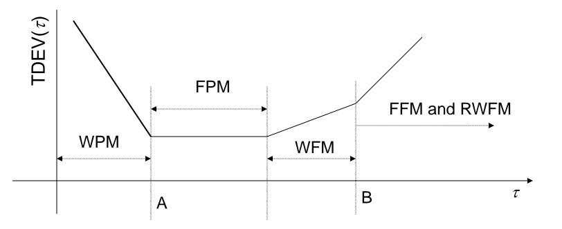
"Phase coherence" for up to A sec.  $\Rightarrow$  Keep PLL time constants less than A sec.
