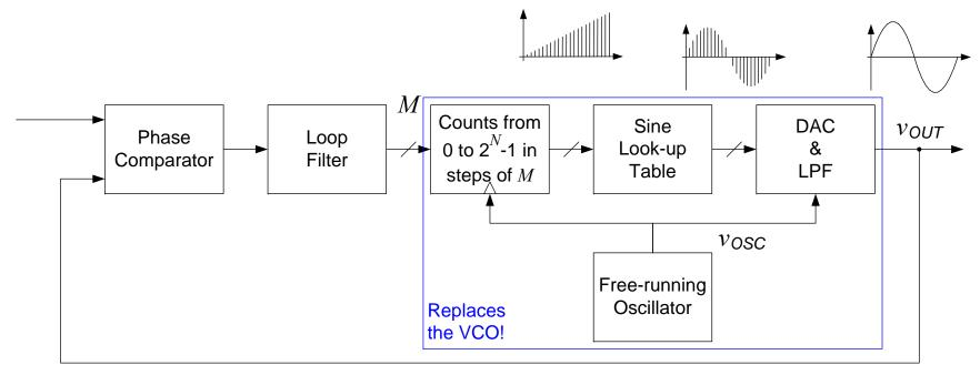
DAC = Digital-to-Analog Converter LPF = Low-pass Filter
