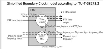
Provides stable reference clock traceable to PRC as reference to PTP
