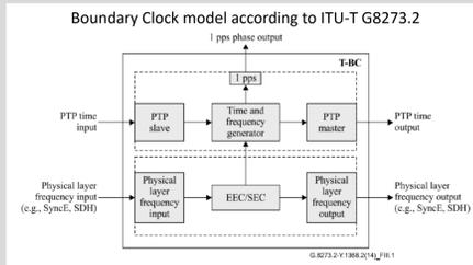
Hybrid mode uses SyncE physical layer frequency to assist PTP
