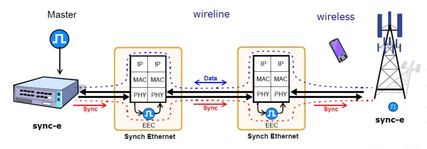
Also referred as **Sync-E**, is an ITU-T standard for computer networking that facilitates the transference of frequency reference signals over the <u>Ethernet physical layer</u>. This signal can then be made traceable to an external clock.
