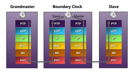
A Boundary Clock has an internal oscillator and can extend the reach, and/or offload slave capacity from the PTP Grandmaster.
