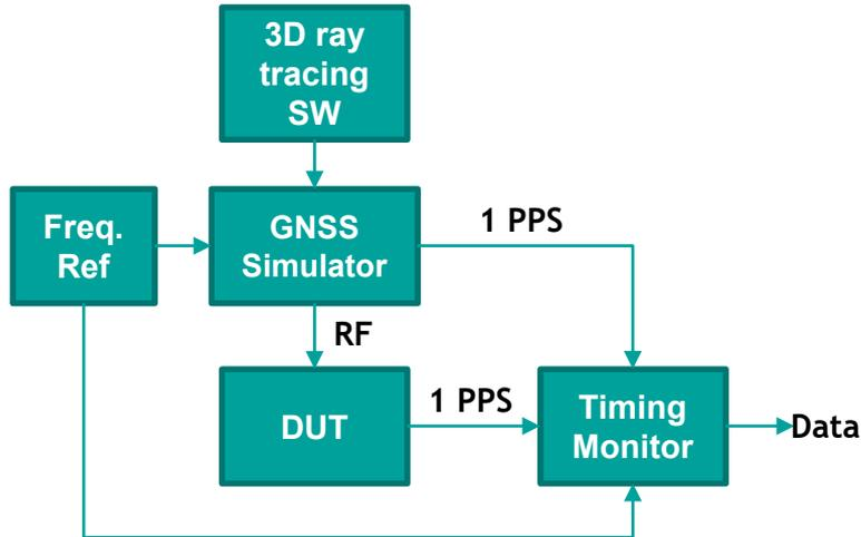
Figure 1: 1 PPS measurement set-up
