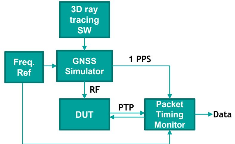
Figure 2: PTP measurement set-up
