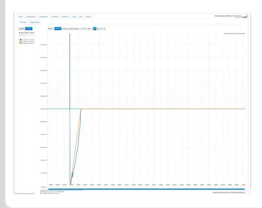
Closing the lid on the notbook suspends the clock. The rapid slewing preserves time ordering but returns the system to correct time (the green line is the primary clock on the client)
