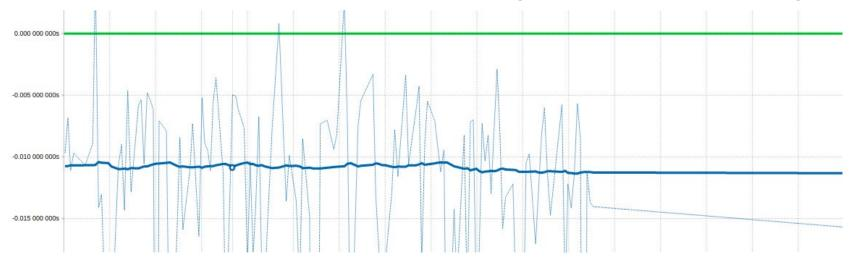
We can track the Internet NTP source pretty well, but it is 10 milliseconds off. A single clock source is impossible to validate from the client. On the other hand, this is external validation of gross time and frequency.
