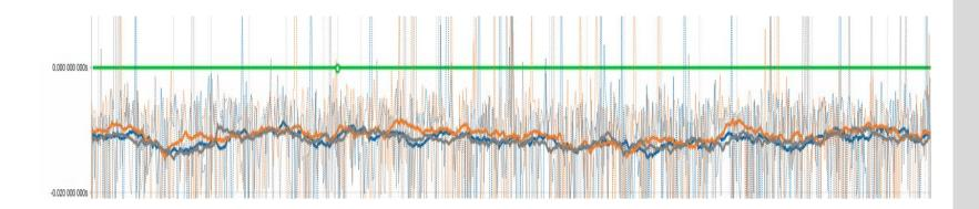
Tracking multiple NTP sources shows they all agree and all have the similar offset. This is probably due to Comcast. But it shows how time provides valuable network connectivity data and limitations of aggregation (you need a smart IT staff, or in this case one with access to smart advice, to distinguish source quality).
