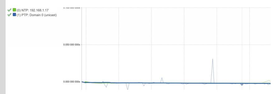
Timekeeper on a notebook computer over wireless (well within the 50 millisecond level regulations are starting to require for "business clocks" on the edge (PTP and NTP feeds validate each other).
