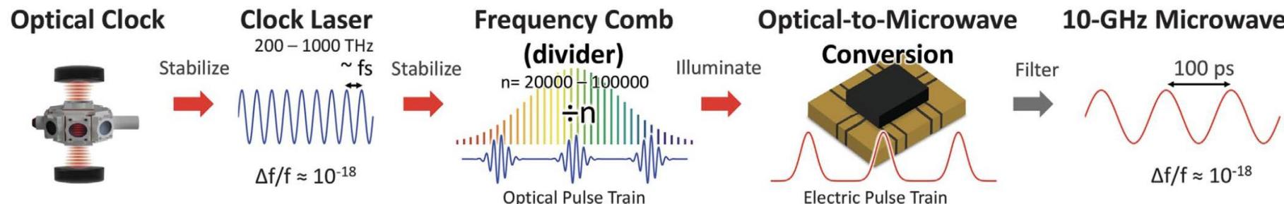
**Coherent optical clock down-conversion for microwave frequencies with  $10^{-18}$  instability, Science 2020 [DOI: 10.1126/science.abb2473](https://doi.org/10.1126/science.abb2473)**
